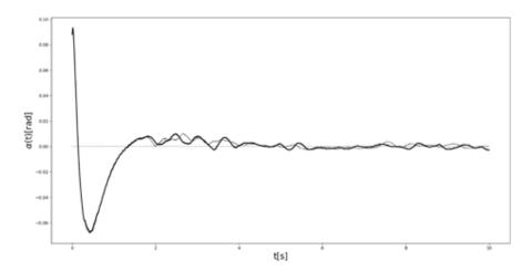
Figure 11 The comparison between stabilization of the pendulum with the compensator (dashed line) and without compensator (solid line) – test on the laboratory stand
