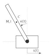
Figure 8 Sketch of the considered control object – the inverted pendulum
