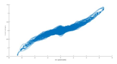
Figure 5 The experimentally-obtained friction characteristic
