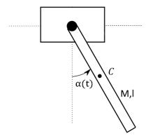
Figure 1 Measurement of pendulum's bar free vibrations
